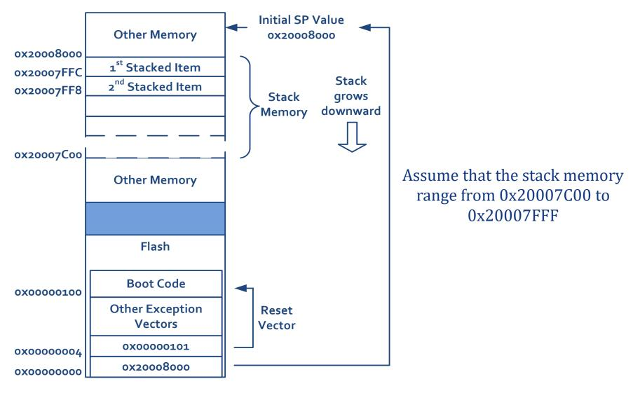
Initial Stack Pointer Value and Initial Program Counter (PC) Value Example
